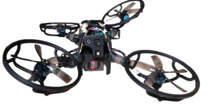
Fig. 1. Flexible “morphy” drone [1], which was infeasible to stabilize with conventional MPC methods. The proposed multi-fidelity controller achieved real-time agile racing performance.
