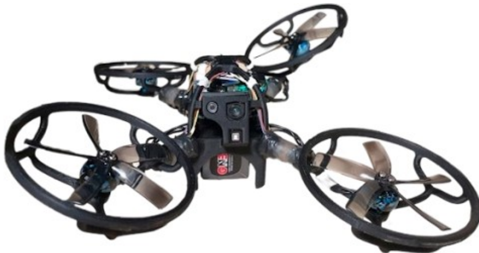
Morphy: compliant quadrotor with passive spring-damper joints [Petrís et al., 2024]
